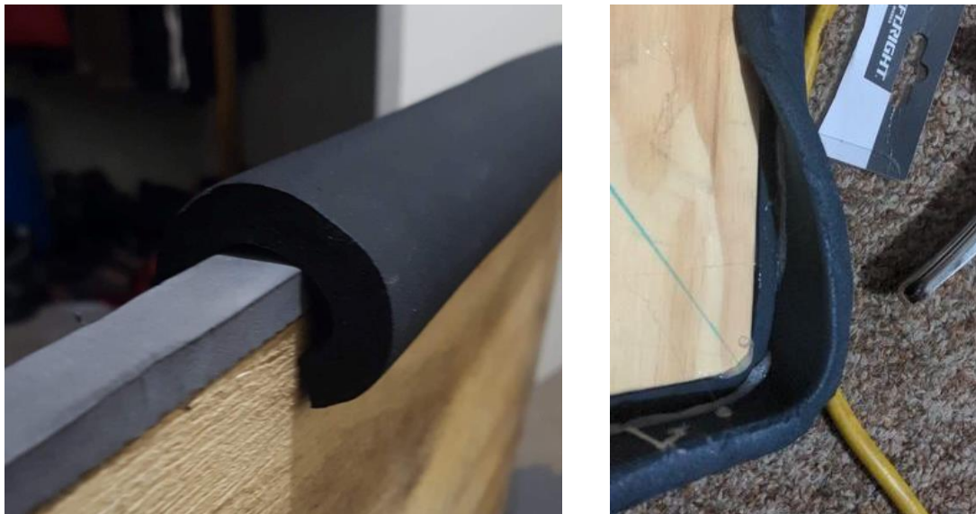
Above are two ways of applying 2 layers of foam to shields
